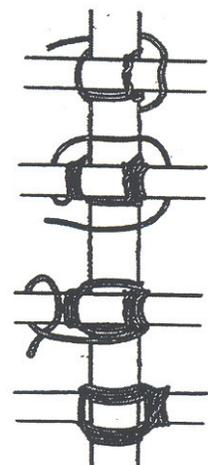
**Diagonal Lashing.** This is used to "spring" two spars together, that is, to lash
